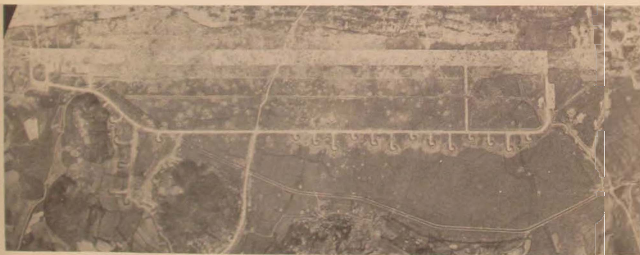
Sunan airfield, featuring a single concrete runway 6700 feet long and 200 feet wide, is in the zone nearest the present battle line. At one time its runway was being extended another 1400 feet, possibly for jet bombers. Its thoroughly bombed runway would probably require a full two weeks of uninterrupted work to be operational.
